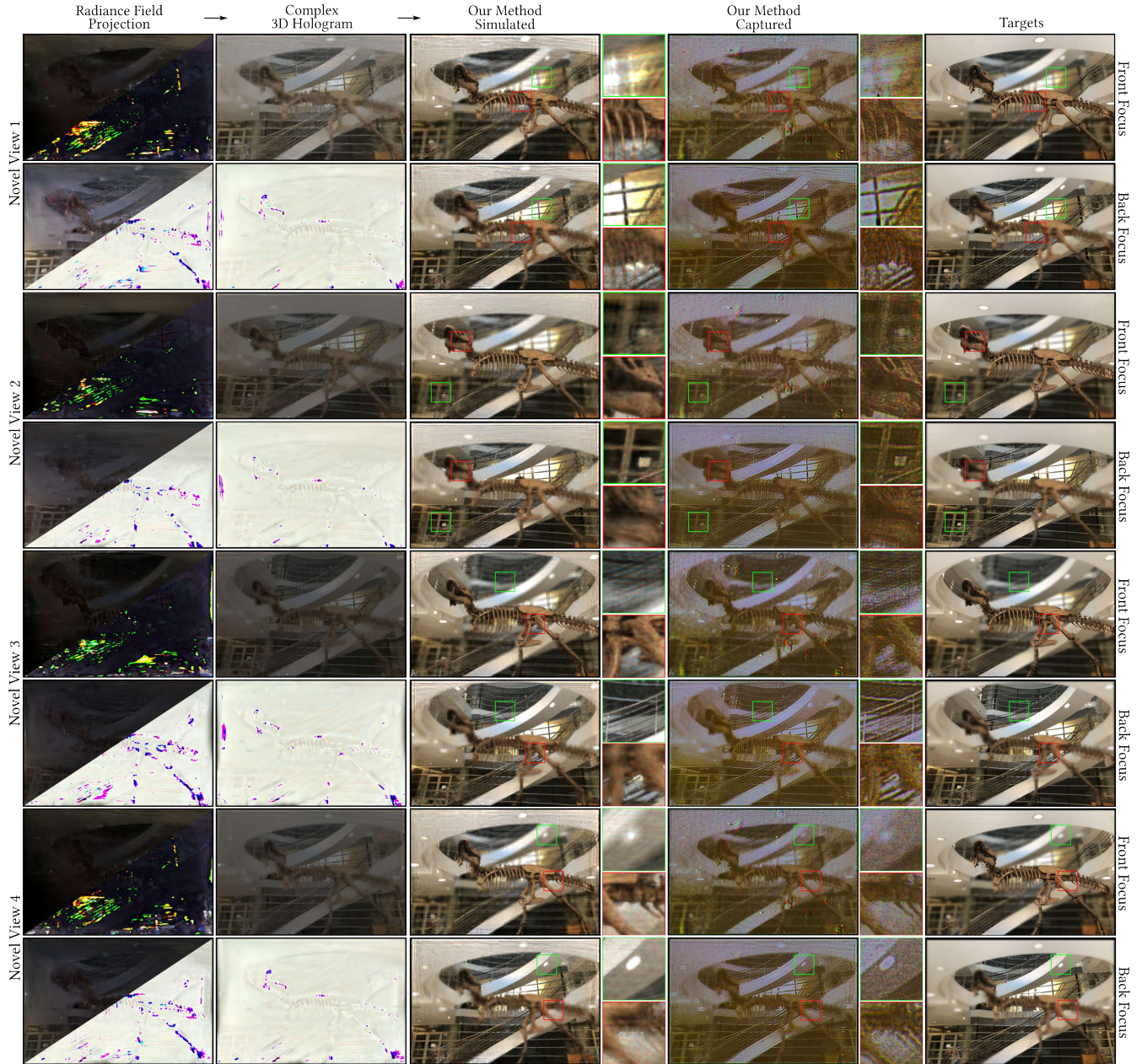
Fig. 14. Extra novel-view comparison of our method on trex scene from the LLFF dataset. The first two columns show the radiance field projections and their rendered complex 3D holograms. The central columns present our method's simulated results and experimentally captured results. The rightmost column displays the target images used as optimization objectives in our method.
