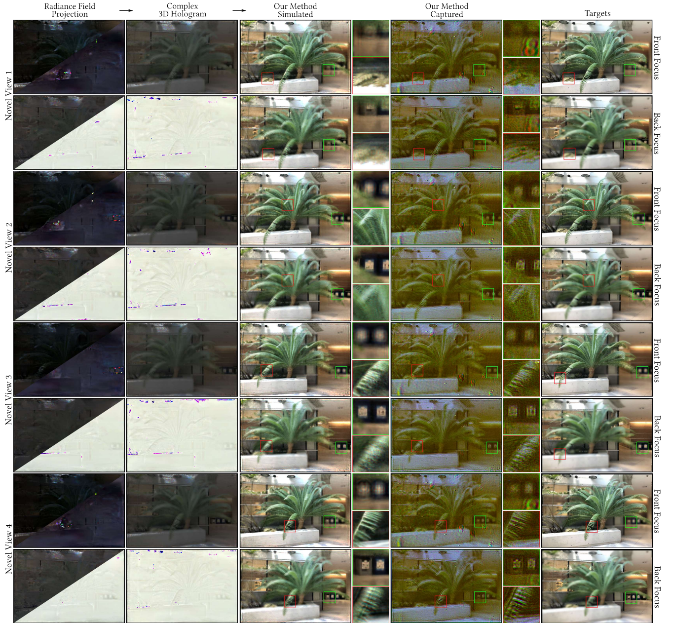
Fig. 13. Extra novel-view comparison of our method on fern scene from the LLFF dataset. The first two columns show the radiance field projections and their rendered complex 3D holograms. The central columns present our method's simulated results and experimentally captured results. The rightmost column displays the target images used as optimization objectives in our method.
