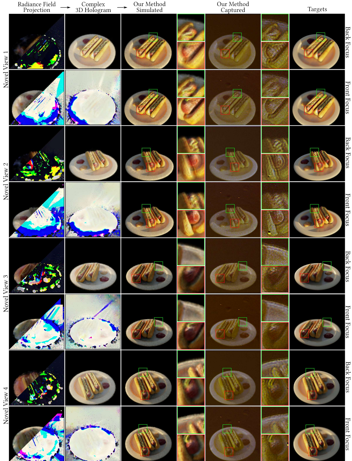
Fig. 11. Extra novel-view comparison of our method on hotdog scene from the NeRF Synthetic dataset. The first two columns show the radiance field projections and their rendered complex 3D holograms. The central columns present our method's simulated results and experimentally captured results. The rightmost column displays the target images used as optimization objectives in our method.
