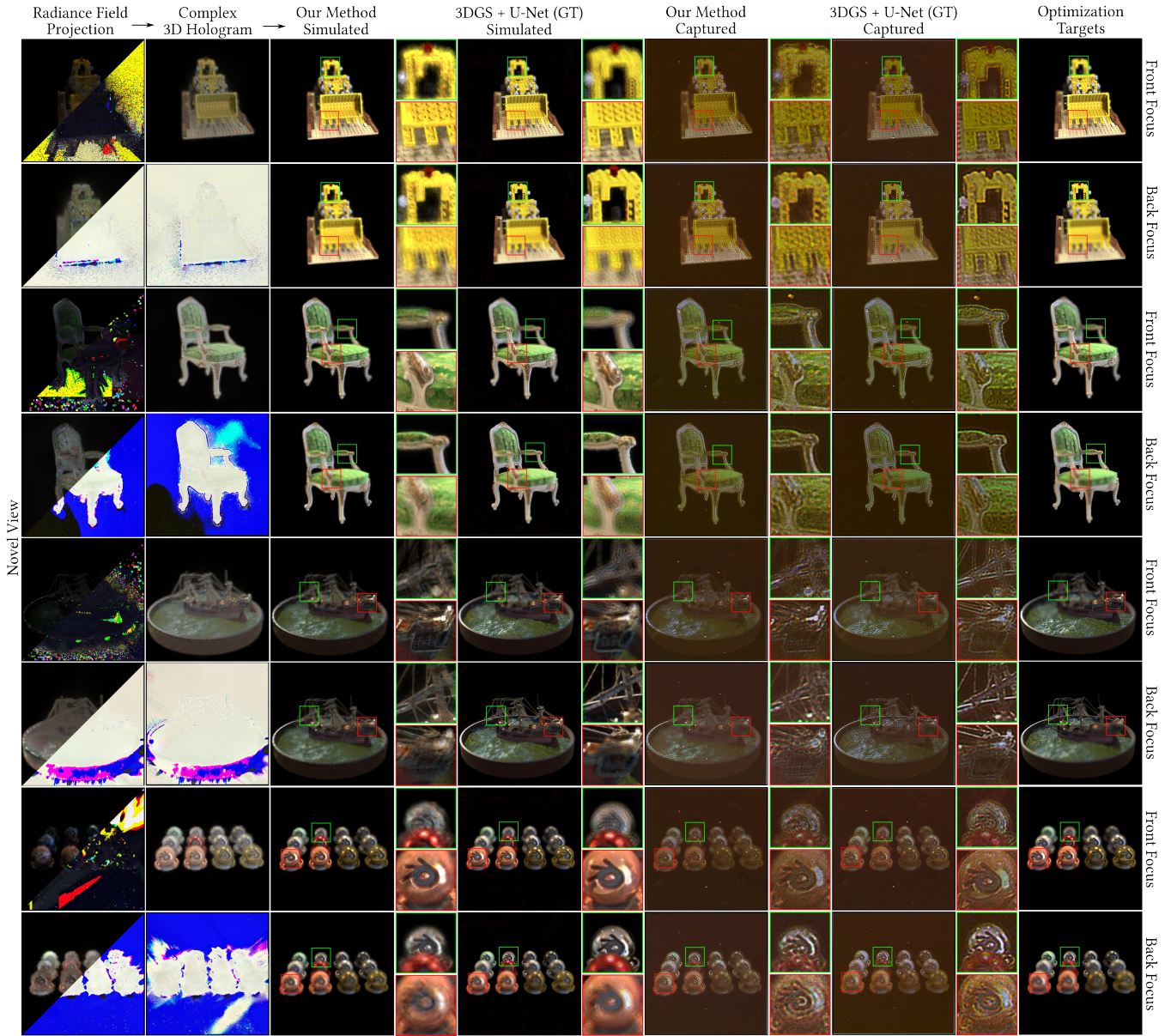
Fig. 8. Novel-view comparison between our method and the 3DGS + U-Net baseline on multiple scenes from the NeRF Synthetic dataset (lego, chair, ship, materials). Here GT represents the Image Quality Ground Truth . The first two columns show the radiance field projections and their rendered complex 3D holograms. The central columns present a side-by-side evaluation of our method’s simulated results and experimentally captured results against the baseline. The rightmost column displays the target images used as optimization objectives in our method.
