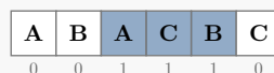
Figure 54: Paint Shop: sequence (A, B, A, C, B, C) with optimal coloring. White = color 0, blue = color 1. 2 color changes (marked ×).
