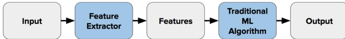
Processing flow for extraction of handcrafted features
